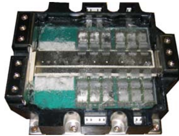
Inside of 900A IGBT module (1400A has the empty spaces filled up)
