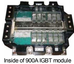
Inside of 900A IGBT module
